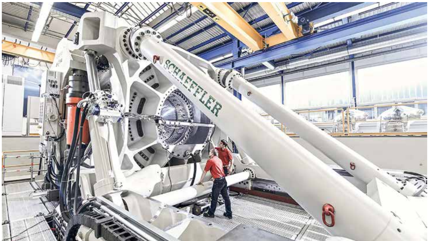
Sensors like the Schaeffler GreaseCheck, Schaeffler LoadSense Pin, and roller set sliding distance sensor are tested and validated on Schaeffler's Astraios large-size bearing test rig
