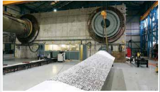
Figure 5: A prototype of the fabric blade undergoing testing.
