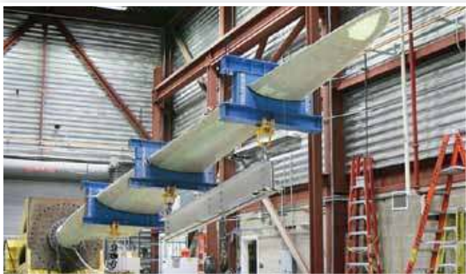
Figure 2: A thermoplastic blade undergoing a simulation of 20 years of use.
