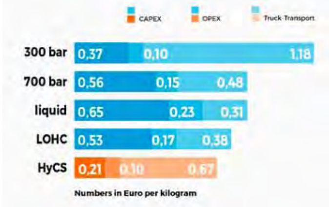
Figure 4: Comparison of Transport costs for different H 2 storage technologies
