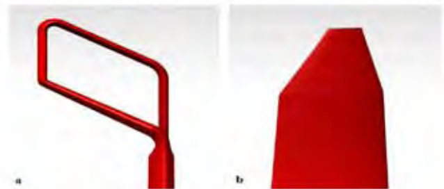
Figure 3: Comparison of spiroid wing-leg (a) and baseline (b) 9
