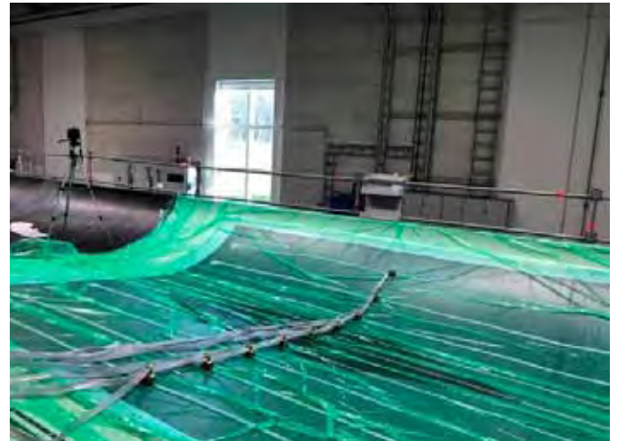
Figure 2: Resin Uptake Test on Optimized Gurit Kit
