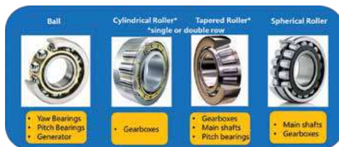
Figure 6: Bearing Types Used at Various Locations in Wind Turbine Systems
