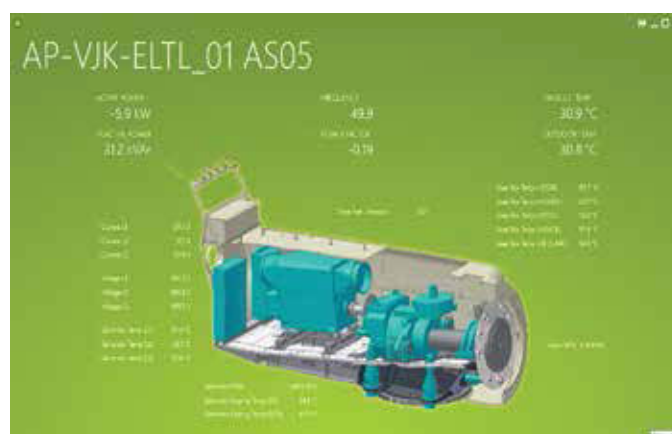
Figure 2: Real Time Monitoring of Wind Turbine Parameters
