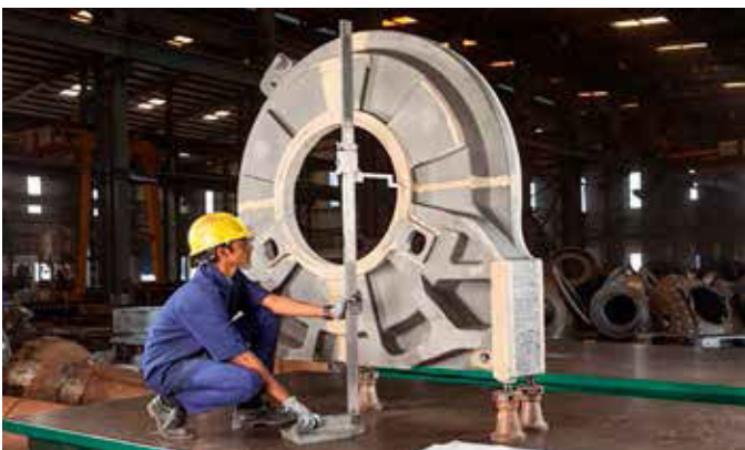
Figure 7: Dimensional Inspection of Wind Gearbox Torque Arm
