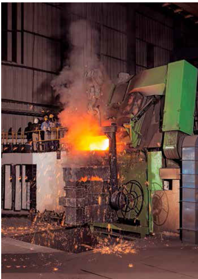
Figure 4: Liquid Metal Tapping
