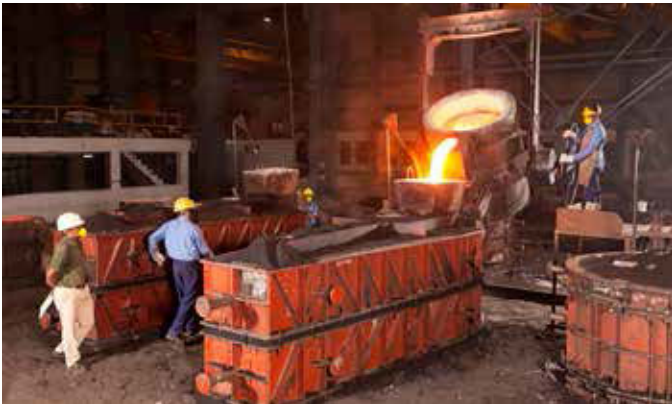
Figure 6: Pouring of Windmill Shaft Casting
