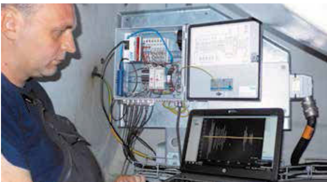
Figure 1: Testing acceleration sensors connected to the PC with analyzer software
