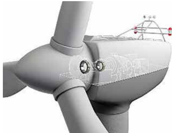
Figure 7: Rotor Shaft Bearing Support in a Wind Turbine
