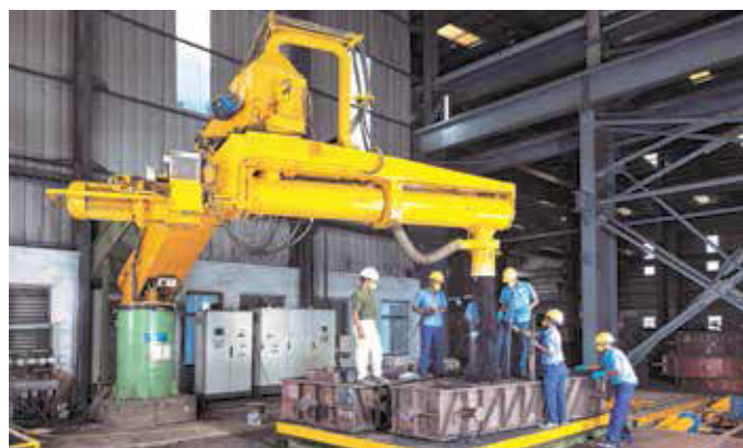
Figure 5: Mould Preparation for Windmill Shaft
