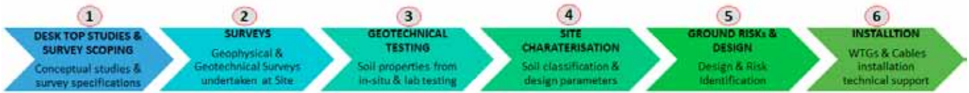
Figure 2: Key stages in an offshore windfarm project where geotechnical consultant’s input is critical
