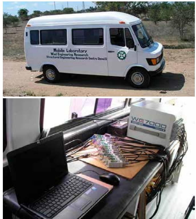
Figure 6: Views of mobile laboratory and DAQ system inside mobile laboratory
