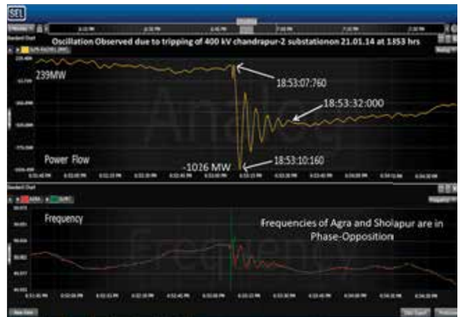
Figure 8: Power Oscillations due to Line Tripping and Associated Recovery with SPS (Courtesy POWERGRID)
