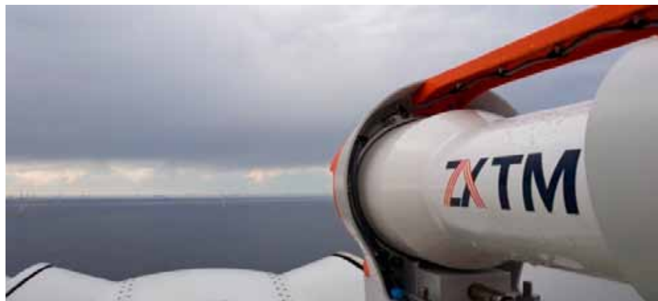
ZX TM Lidar installed at Galloper Wind Farm for RWE Power Performance Test of SGRE 6MW
