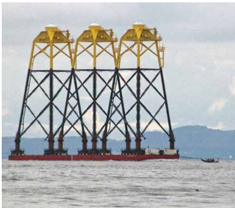
Wiking offshore wind farm - Jacket Foundations
