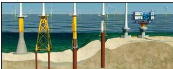
Figure 2: Illustration of OWF Foundations Designed by COWI. From left: Thornton Bank Concrete Gravity based, Wikingier Jacket (Preliminary Stage), Two Times London Array Monopile, Nysted WTG and Rødsand 2 Offshore Substation Concrete Gravity Based
