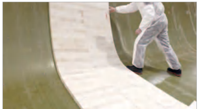
Figure 5: Opticore software enables kitting of core materials to reduce waste and minimize production time
