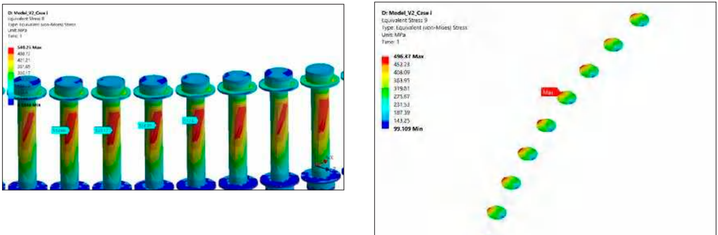
Figure 9: Stress observed at Bolt Joint
