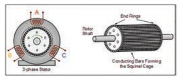
Figure 1: Squirrel Cage Induction Generator<sup>2</sup>
