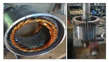
Figure 3: Doubly Wound Stator and Specially Designed Rotor of 3.5 kW BDFIG Prototype Developed at Amrita Vishwa Vidyapeetham, Coimbatore
