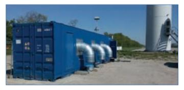
Figure 4: FRT Container of Deutsche WindGuard
