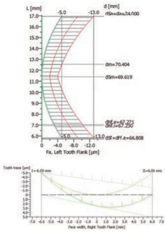
Figure 3: Profile and Lead modification curves thru LTCA Analysis
