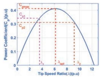
Figure 2: Typical Wind Turbine Characteristics
