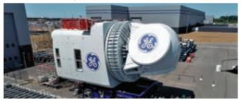
Figure 5: Nacelle of a 12 MW Wind Turbine<sup>7</sup>
