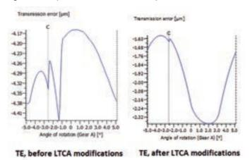
Figure 4: Transmission Error Analysis
